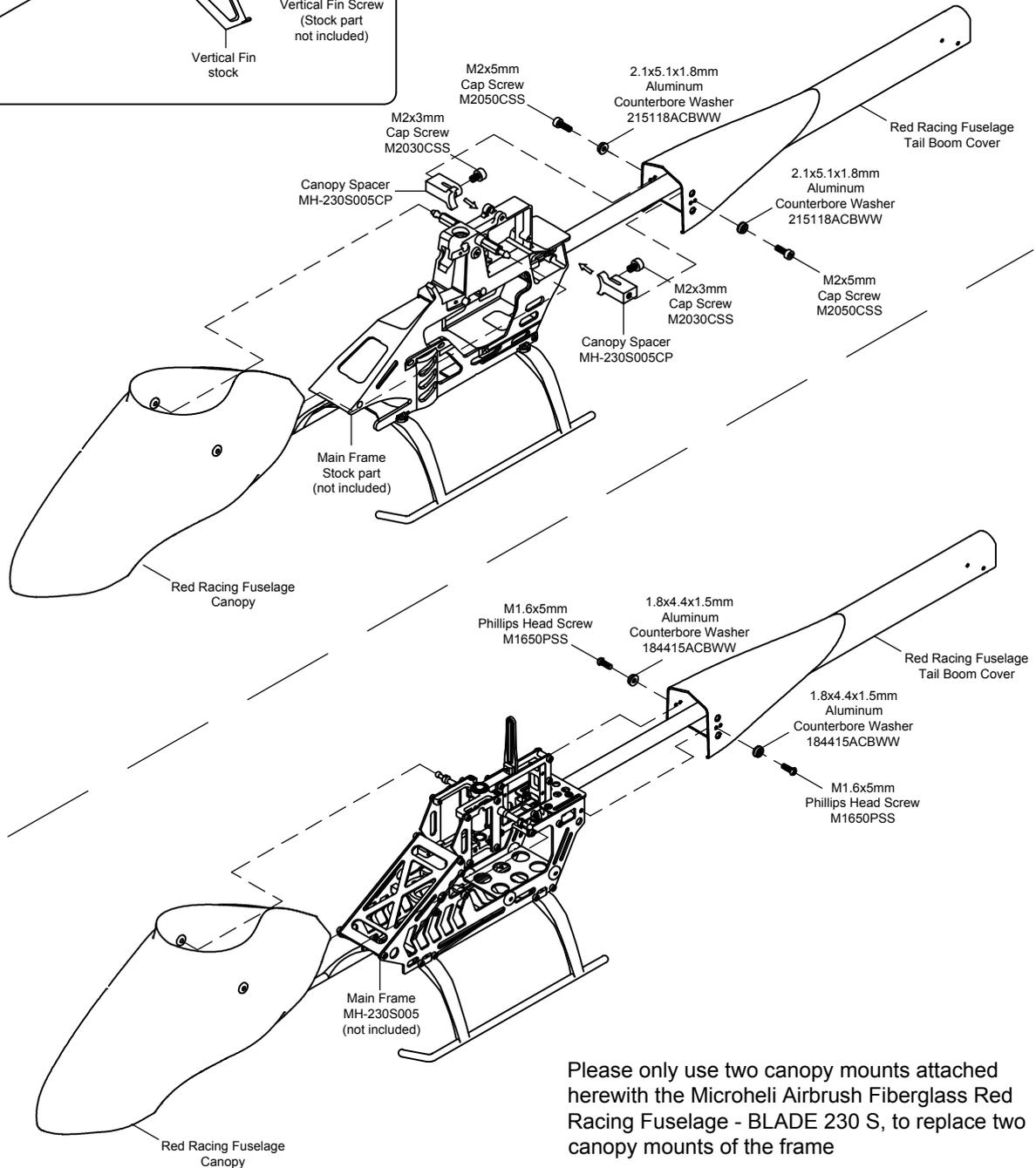
Please only use two canopy mounts attached herewith the Microheli Airbrush Fiberglass Red Racing Fuselage - BLADE 230 S, to replace two canopy mounts of the frame
